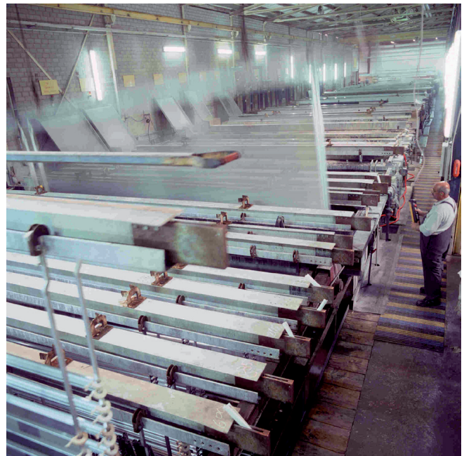
Hot seal bath: the sealing is always the concluding step in the eloxal process
